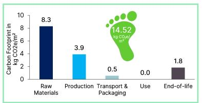
The renowned institution TÜV Rheinland (Germany) has certified the carbon footprint of Heliatek's organic solar film HeliaSol to be 14.52 kg CO<sub>2</sub>e/m². By means of a Life Cycle Assessment (LCA) all environmental impacts were evaluated from acquisition of raw materials over the production and use up to end-of-life treatment including all transportation effects.
